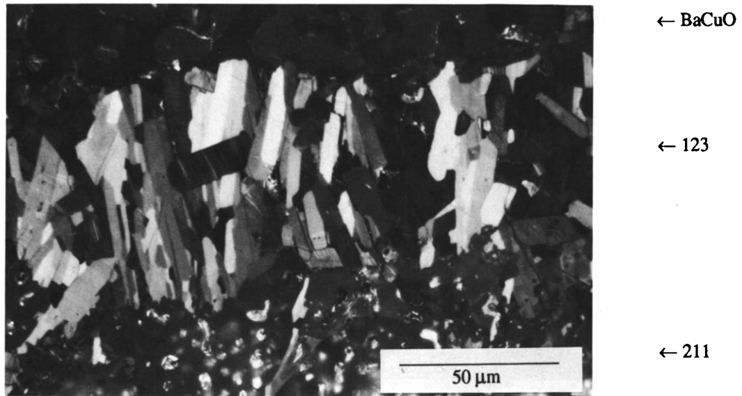
Figure 2. Optical micrograph of the cross section of a 123 layer grown during 5 h on a substrate sintered 30h at 1150°C and 30h at 1210°C.
